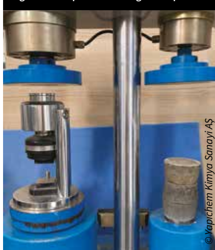
Figure 5: compressive strength test press
