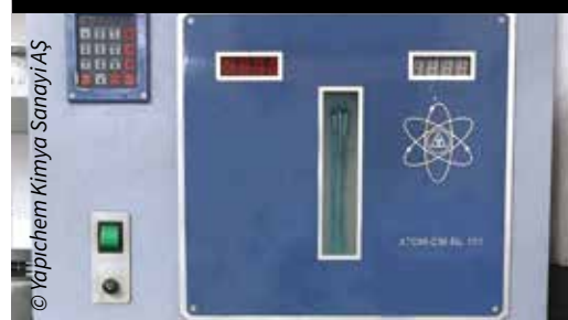
Figure 1: the specific surface area of the OPC used in the study was carried out with Blaine air permeability apparatus
