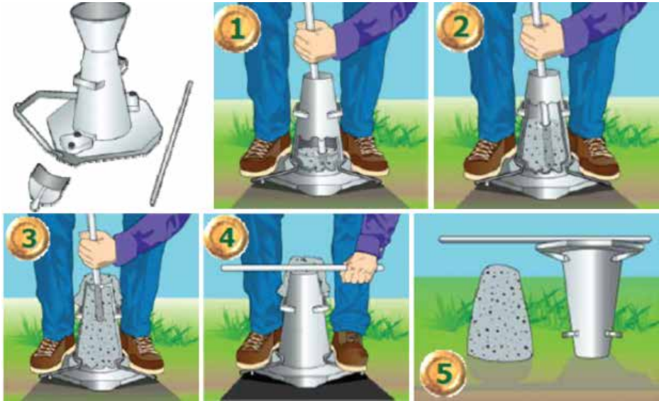
Figure 6 Slump test
