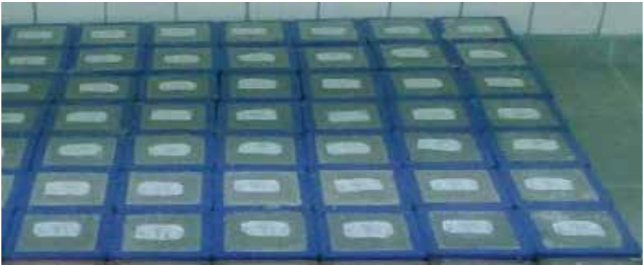
Figure 8 Concrete sample molds
